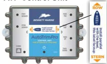
The ATP Control Unit is the sensor and processor for the ATP system. The ATP Control Unit contains an accelerometer, gyroscope, and an electronic compass that sense the position of the boat and the accelerations and decelerations that the boat is moving through. **The ATP Control Unit must be properly oriented on the boat to correctly interpret acceleration and deceleration.** The ATP Control Unit activates the hydraulic pumps that run the trim tabs.
