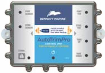
The ATP control unit must be mounted horizontally and parallel with the keel of the boat. The label indicates with an arrow which end should be oriented towards the bow of the boat. The location of the ATP control unit within the boat is not critical, but the orientation of the
