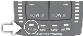
display should show the actuators position as the actuators retract.
