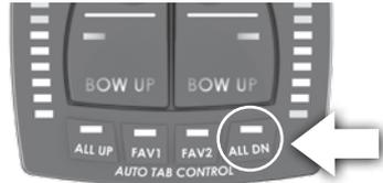
8. Press the ALL UP button. The actuators should retract, and the display should show the actuators position as the actuators retract.
