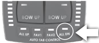
actuators should extend, and the display should show the actuator position as the actuators deploy
