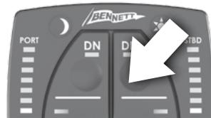
port actuator should extend. If the port actuator does not extend, or the stbd. actuator extends instead of the port actuator, refer to the troubleshooting section.
