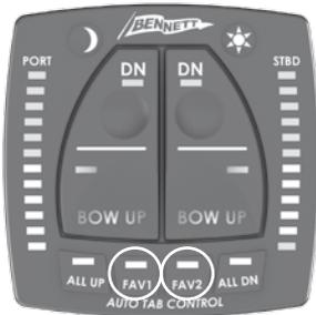
start automatic operations, the unit must have the FAV position set (see "Setting a Favorite Position" on page 37), and it must have the three set-up
